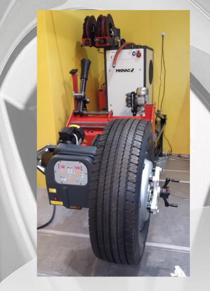
From the other side the unit become a wheel balancer for truck, buses, light truck and passanger wheels.
