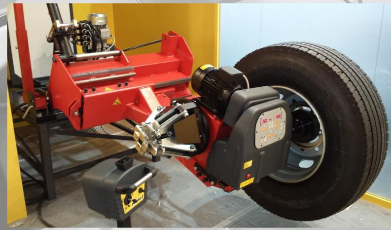
From one side the unit is capable to mount and dismount all kind of truck, buses, light truck and passanger wheels.
