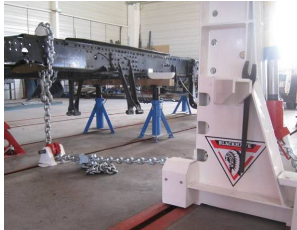
Pulling Down (Low Height)
