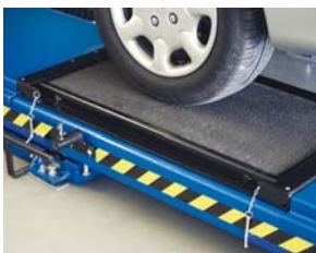
Slip plate, rotational movement +/- 5°, lateral movement +/- 50 mm (Option)
