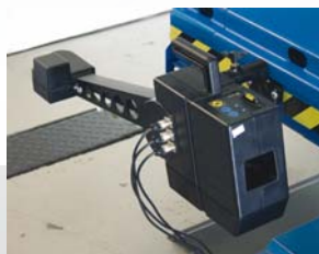
Precision holder for measuring tools and test position control system MKS (Option)
