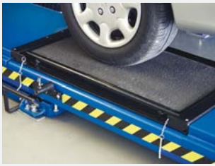
Slip plate, rotational movement +/- 5°, lateral movement +/- 50 mm
