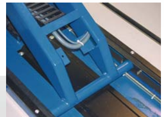
Cables and hoses ideally protected by installation inside scissors tubes
