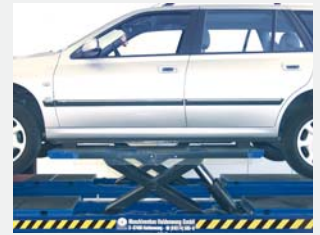
Wheel-free jack raises complete vehicle when positioned on runways
