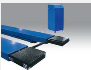
Axle play detector with cable hand lamp
