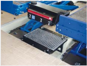
Pneumatic floor cover for strip foundation
